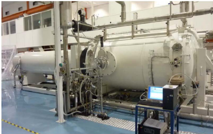
Thermal-vacuum chamber equipped with the solar simulator
